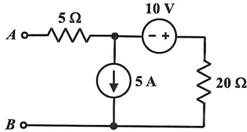
Determine the Norton equivalent circuit with respect to terminals *A* and *B*.
